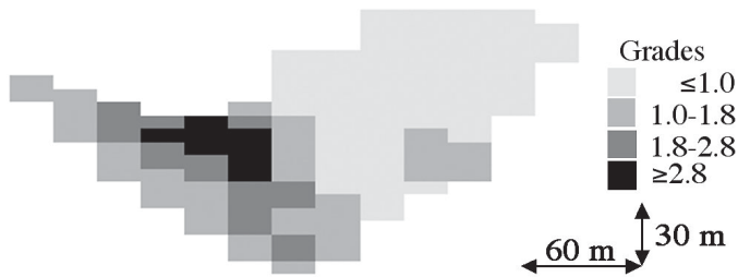
Figure 1 — Grade distribution of gold on a south-north cross-section of the orebody model.
