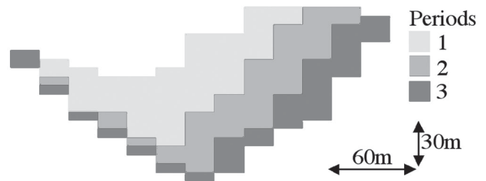
Figure 2 — South-north cross-sectional view for the optimal schedule showing the three scheduled periods of blocks
